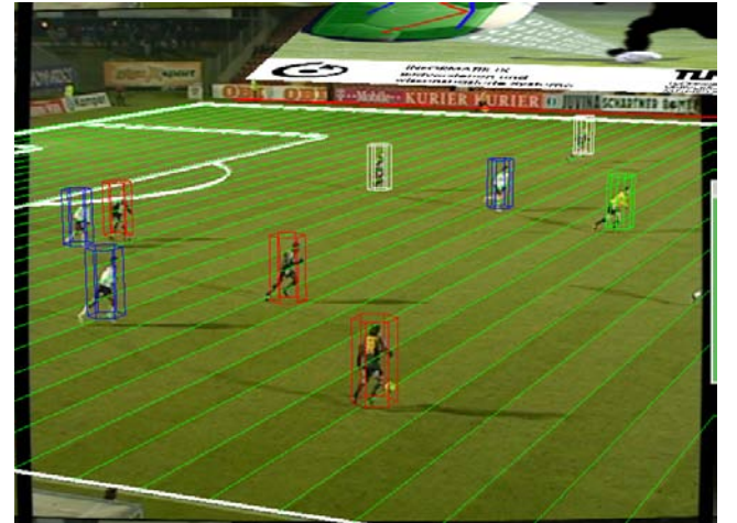
Figure 2: Output of the visual perception. The players and the ball in the camera view are detected. The players are labelled with respect to the team they belong to. For each player, the referee, and the ball the \langle x, y \rangle position is estimated.
