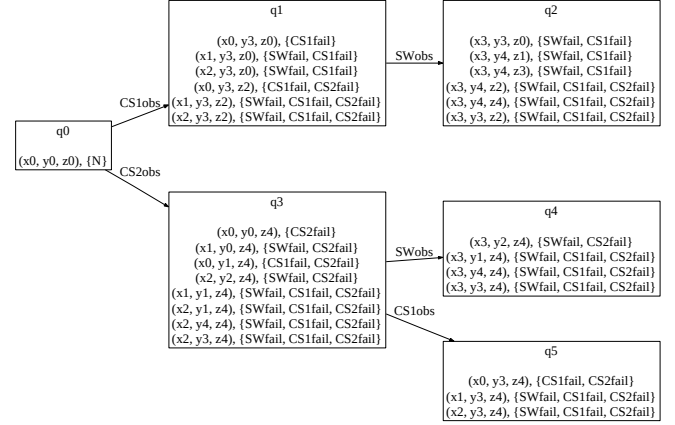
Figure 2. (Part of the) diagnoser for the example shown in Figure 1.
