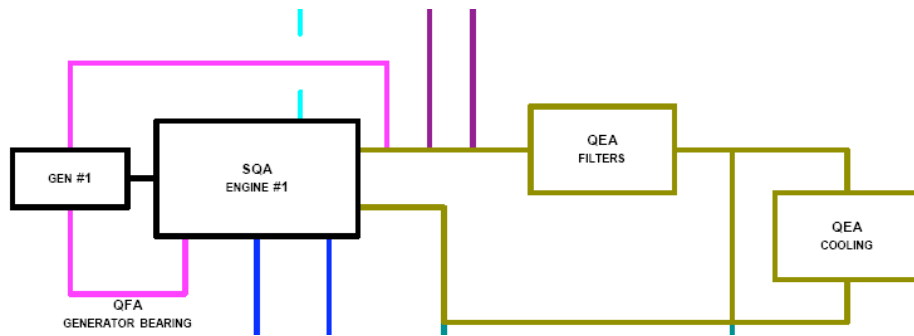
Fig. 2. A part of one of the block diagrams. The concepts in this block diagram detail the lube oil system in a power plant.
