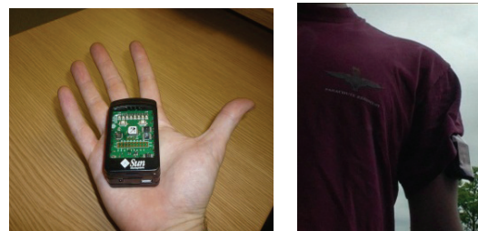
Fig 1. SunSPOT (on a palm and attached to the arm; size 63x38x25mm)
