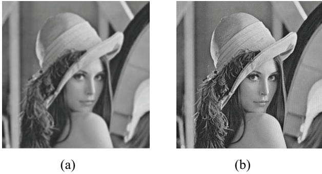
Figure 10. (a) The received degraded Lena, PSF size: 7 \times 7 , \sigma : 3.5. (b) Estimation image and PSF Size: 7 \times 7 , \sigma : 3.5591
