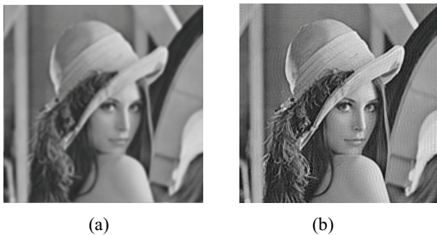
Figure 12. (a) The received degraded Lena, PSF size: 9 \times 9 , \sigma : 4. (b) Estimation image and PSF Size: 9 \times 9 , \sigma : 4.2907
