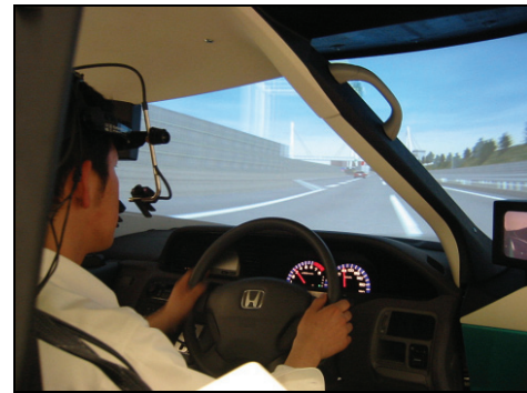
Figure 3. Driver wearing eye tracking system in driving simulator
