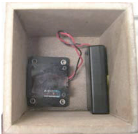
Figure 6. Wireless accelerometer built in a building block
