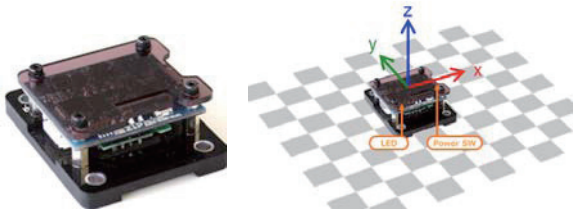
(a) Wireless accelerometer (b) Sensing direction
