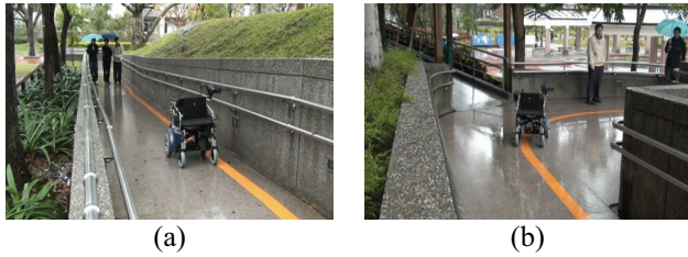
Figure 13. Actual testing environment (rainy day), (a) path of straight paint line, (b) path of curve paint line
