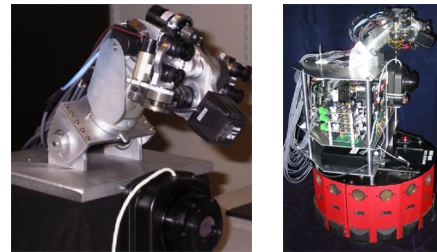
Figure 1: (Left) The M4 Macaco robot, designed to resemble a dog's head. (Right) The M4-Macaco robotic head and processing hardware assembled to a Magellan mobile platform.
