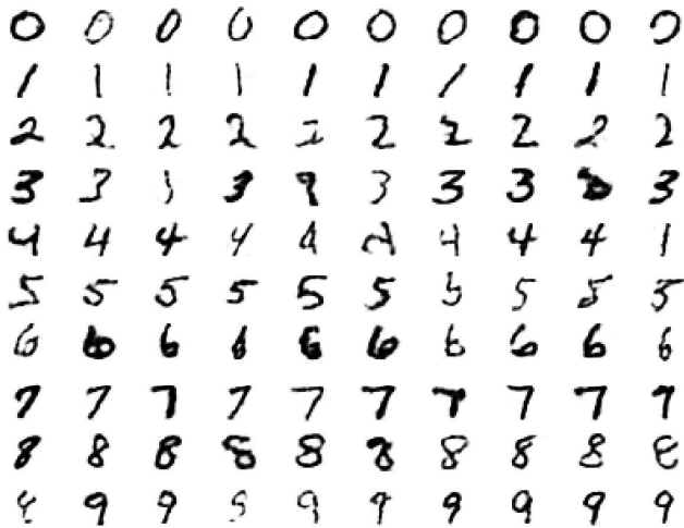
Figure 9: Each row shows 10 samples from the generative model with a particular label clamped on. The top-level associative memory is run for 1000 iterations of alternating Gibbs sampling between samples.
