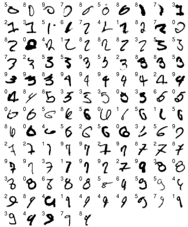
Figure 8: The 125 test cases that the network got wrong. Each case is labeled by the network's guess. The true classes are arranged in standard scan order.
