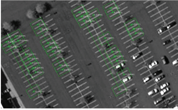
Figure 2: An illustrative example image is shown. The low-level analysis produces the estimated parameters and a set of canonical parking spots templates that are depicted by (green) rectangular patches around their centroids. There are 55 canonical parking spots obtained in this example. Viewed best in color.
