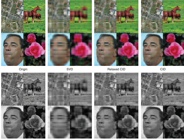
Figure 1: Image reconstruction using SVD, CID, and Relaxed CID on color images (top) and gray level images (bottom). Four images are from diverse data source (see §4.1). For SVD, k = 4 ; parameters for CID and Relaxed CID are set such that all methods use the same storage. The reconstruction errors of SVD, Relaxed CID, CID are 2.98%, 2.22%, 1.51% for color images, and 6.27%, 4.43%, 2.95% for gray level images. CID has the best results and Relaxed CID is also better than SVD.
