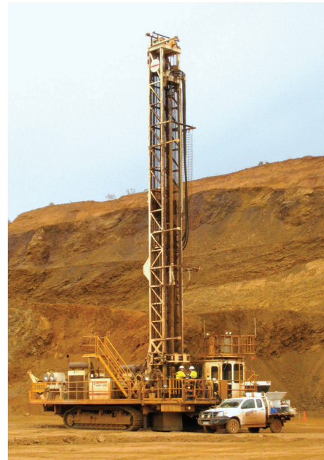
Figure 3: Drill-rig used to collect MWD data.
