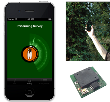
Figure 8: Prototype app interface showing the real-time feedback presented to the user during a 60 second survey, indicating the detection of a cicada song, and the electronic cicada that replicates the sound of the cicada, used for user testing.
