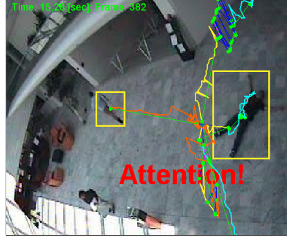
Fig. 2. A logical inference has found a possible case of a sudden attack in the graph of blob trajectories. All probable participants of the conflict are marked by yellow rectangles. The tracks are depicted by lines.
